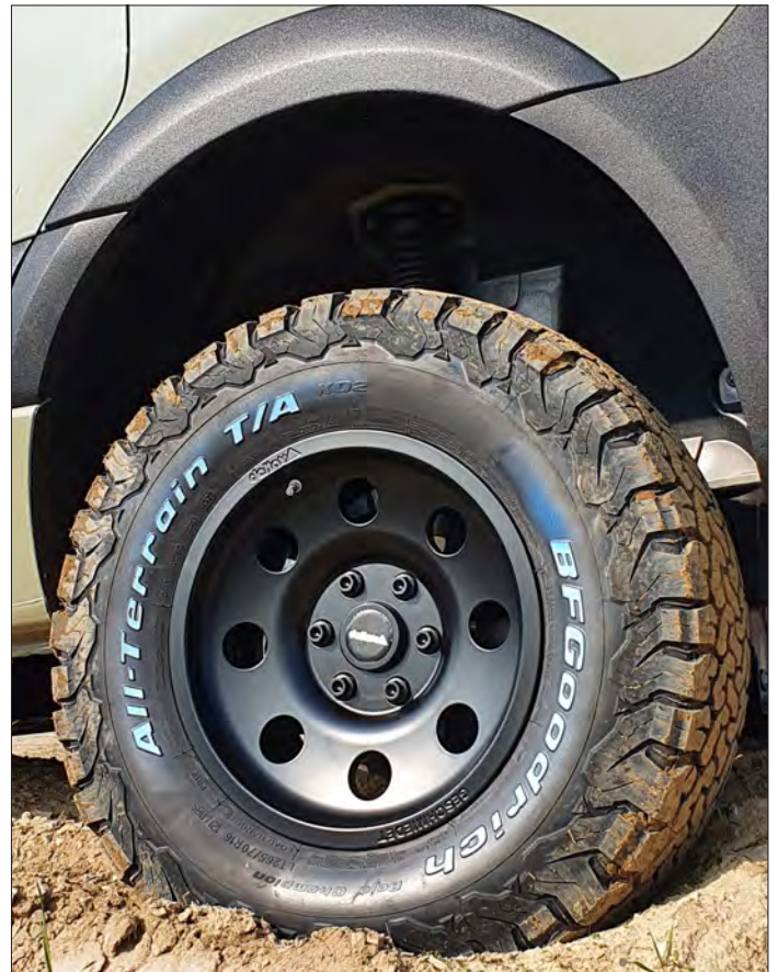
Felge/Wheel Legacy Forged 16x8 Reifen/Tire 265/70-16 BFGoodrich
